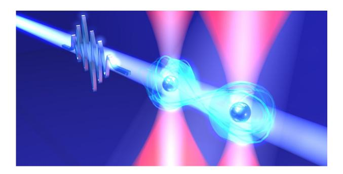
Fig. 1. Conceptual diagram of the world's fastest two-qubit gate. Two atoms captured in optical tweezers (red light) with a separation of a micrometer are manipulated by a ultrafast laser pulse (blue light) shone for only 10 picoseconds. Credit: Dr. Takafumi Tomita (IMS)
