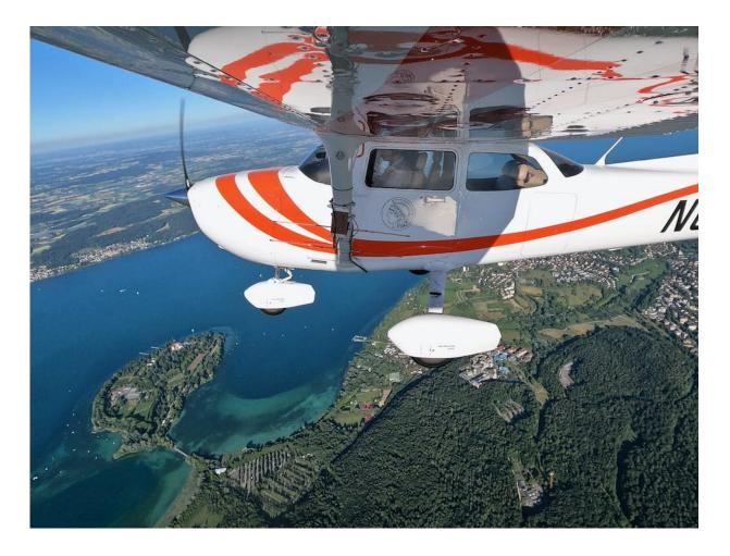
A Cessna aircraft was fitted with antennas and flown in circles in the air to home in on the radio signal. Credit: Max Planck Institute of Animal Behaviour, Author provided
