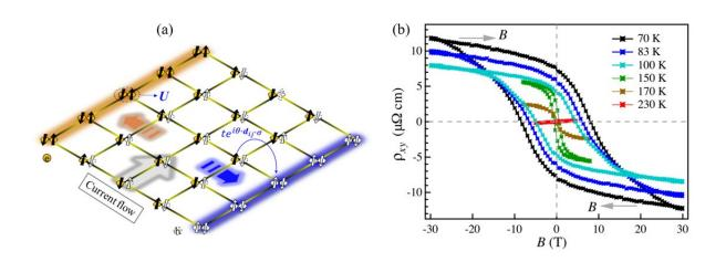
(a) Schematic of anomalous Hall effect in the intermediate coupling regime; (b) Magnetic field dependent Hall measurements at different temperatures. Credit: Hao Lin
