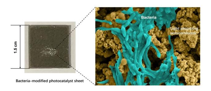
Photocatalyst sheet containing light-absorbing particles and bacteria. Credit: Northumbria University
