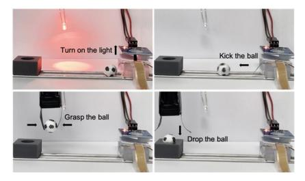
Various actuation motions of low voltage actuator. Credit: POSTECH
