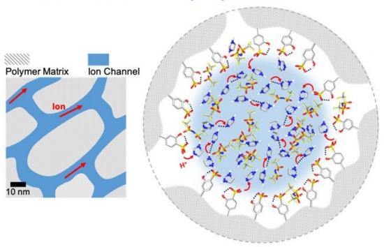
Schematic diagram of ion channel formation inside the polymer electrolyte. Credit: POSTECH
