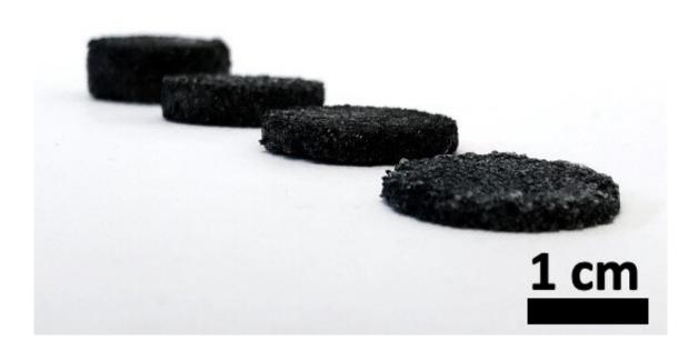
Sponge electrodes, seen here in a variety of thicknesses, use sugar cubes as templates. Credit: Adapted from *ACS Nano*
