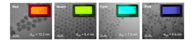
TEM images for the particle sizes of red, green, cyan, and blue QDs used for the device fabrication and charge transport simulation. dQD is the average diameter of the QD nanoparticles. Insets are the snapshots of EL-driven monochromatic red, green, cyan, and blue QD-LED devices fabricated by the transfer printing technique. The size of the fabricated device is  $3.0 \times 1.5 \text{ mm}^2$ . Credit: *Nature Communications* (2022). DOI: 10.1038/s41467-022-31853-9
