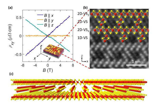
Discovery of a new superlattice structure exhibiting the anisotropic Hall effect. (a) Anisotropic Hall effect. (b) Scanning transmission electron microscopy (STEM) cross sectional image of 2D-VS2/1D-VS superlattice structure. (c) Schematic model of the 2D/1D hybrid superlattice. Credit: Y.C. Lin
