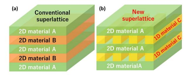
(a) Conventional superlattice structure model consisting of different 2D materials. (b) Newly discovered superlattice structure model consisting of twodimensional (film-like) and one-dimensional (chain-like) materials. Credit: Y.C. Lin
