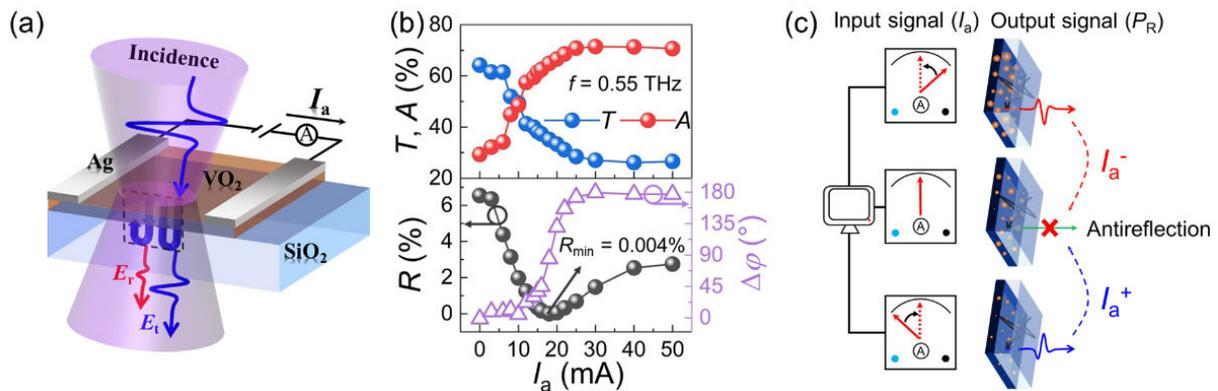
(a) Schematic diagram of active THz electro-optic modulator based on VO<sub>2</sub> film. (b) Experimental transmission (T), reflection (R), absorption (A) and reflection phase shift ( $\Delta\varphi$ ) as a function of applied electric current at 0.55 THz. (c) Schematic diagram of smart THz manipulation. Credit: Ren Zhuang
