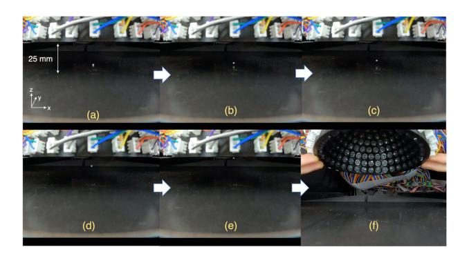
Photograph highlighting the picking up of a particle on the rigid stage: (a) successful picking up; (c)–(d) upward motion; and (f) successfully maintaining the particle. Credit: *Japanese Journal of Applied Physics* (2022). DOI: 10.35848/1347-4065/ac51c4
