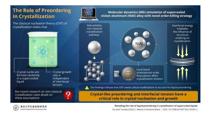
Molecular dynamics simulations of a supercooled nickel–aluminum alloy reveal that crystal-like preordering and interfacial tension are important in crystal nucleation and growth, highlighting a critical gap in classical nucleation theory. Credit: Hajime Tanaka from University of Tokyo
