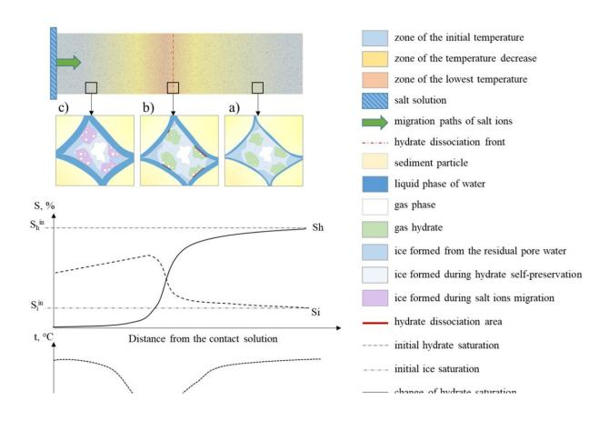
Temperature changes caused by salt migration in frozen sand containing metastable gas hydrates, accompanied by phase transitions of pore moisture and variations of ice and hydrate saturation along the sample. Credit: *Geosciences* (2022). DOI: 10.3390/geosciences12070261
