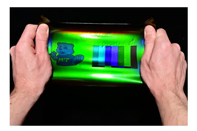
By applying a 19th-century color photography technique to modern holographic materials, an MIT team has printed large-scale images onto elastic materials that when stretched can transform their color, reflecting different wavelengths as the material is strained. Credit: Mathias Kolle et al
