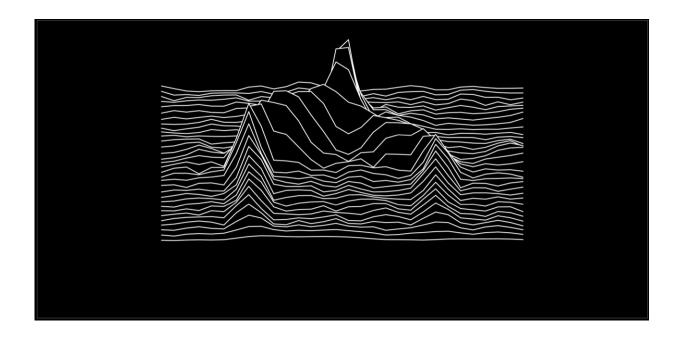
Experimental frequency spectra of photons leaking from the cavity. As time progresses (top to bottom), the system evolves from a single configuration into two distinctly different ones, reflected in the splitting into two peaks. Credit: ETH Zurich / Alexander Baumgärtner
