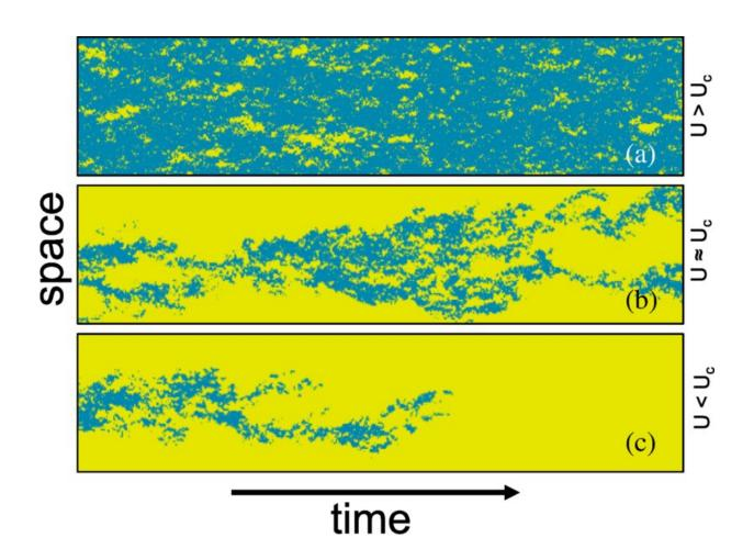
Space-time plot of laminar-turbulent transition as a function of U (i.e., Reynolds number) generated by the PP model in quasi-1D Taylor-Couette flow. Turbulence (in blue) is represented by the prey density B, generated by Monte Carlo simulation on a 2D lattice of size  $20 \times 3000$  (a) below the critical point U=0.0135, (b) at the critical point U=0.01425, and (c) above the critical point U=0.0165. Yellow represents the laminar phase locally unoccupied by the prey.
