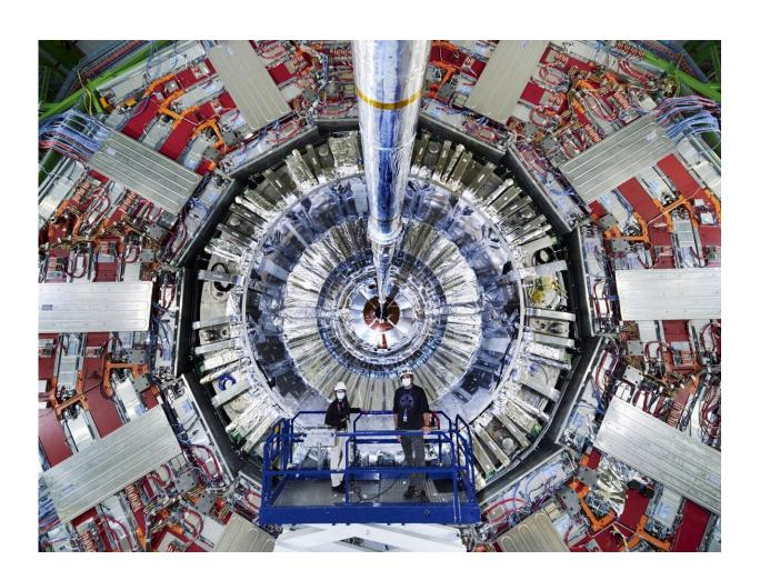
The CMS detector completed several upgrades during a three-year-long shutdown to prepare for the current physics run at the LHC. Additional upgrades planned for installation during the next long shutdown will prepare the experiment for the High-Luminosity LHC. Credit: Samuel Joseph Hertzog, CERN
