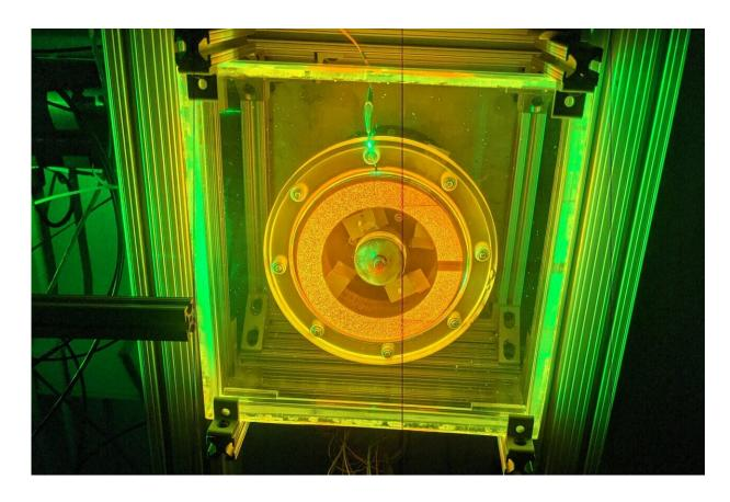
The setup allowed the researchers to reconstruct the flow by tracking the motion of millions of suspended fluorescent particles. Credit: Photo: Michael Schatz
