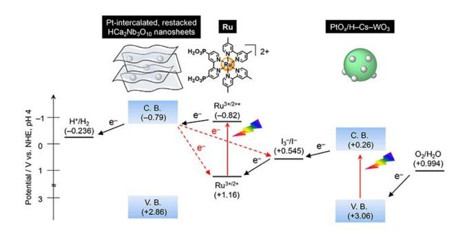
The oxygen evolution catalyst efficiently reduces the concentration of the  $I_3^-$  ions and changes to the hydrogen evolution catalyst prevent electron back transfers (dotted red lines) and prioritize electron transfer to produce hydrogen (solid black lines). Credit: Tokyo Institute of Technology
