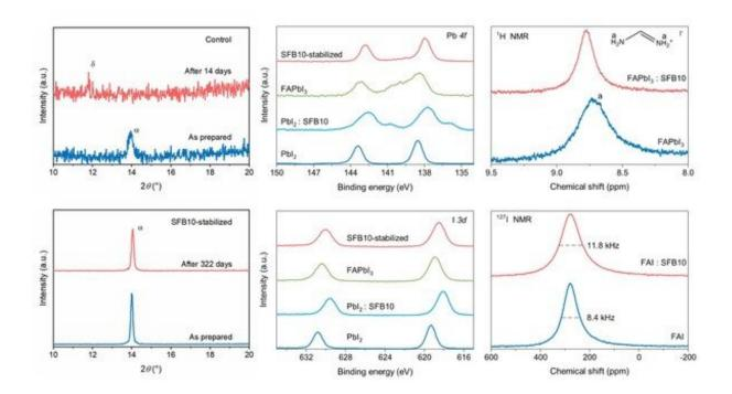
Figure 3: Structural and chemical analyses of the perovskite samples. Credit: *Nature Photonics* (2022). DOI: 10.1038/s41566-022-01046-3
