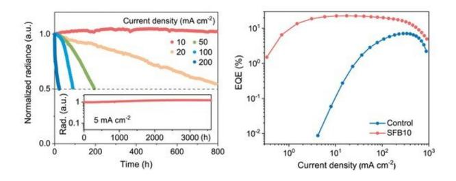
Figure 2: Long-term operation and accelerated aging experiments of the perovskite LEDs (left panel); external quantum efficiency data of the stabilized and untreated devices (right panel). Credit: *Nature Photonics* (2022). DOI: 10.1038/s41566-022-01046-3
