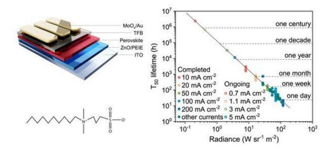
Figure 1: Structure of the perovskite LED (upper left panel); structure of the dipolar molecular stabilizer, SFB10 (lower left panel); device T50 lifetimes versus the optical power output (radiance) of the perovskite LEDs (right panel). Credit: *Nature Photonics* (2022). DOI: 10.1038/s41566-022-01046-3
