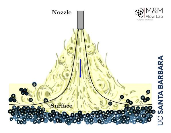
The nozzle (top) creates a flow of turbulent air that interrupts cohesionbetween particles (below) and the surface, leading to erosion and transport of the particles. Credit: UC Santa Barbara
