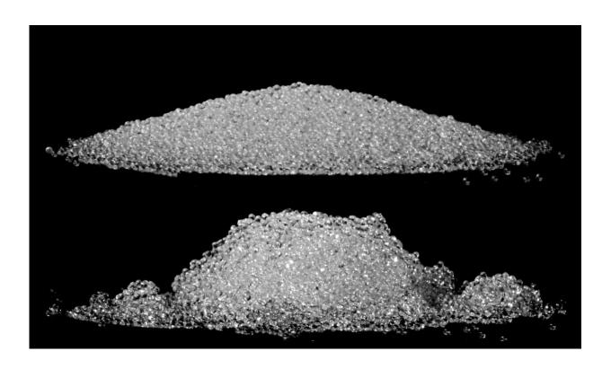
The polymer-covered spherical glass beads used in the experiments. The grains at the top havea very thin coating and no cohesion; those at the bottom have a much thicker coating and arecohesive. Credit: UC Santa Barbara
