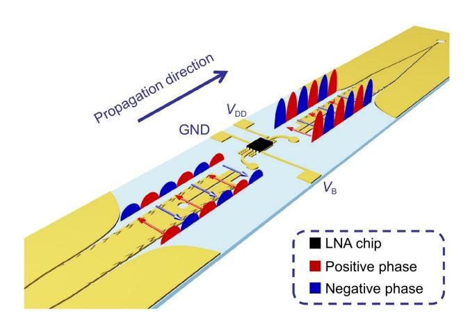
Schematic diagram of the whole amplifier-integrated OMM. Credit: *Opto-Electronic Advances* (2022). DOI: 10.29026/oea.2022.210119
