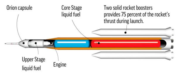
A cutaway of the Space Launch System or SLS.
