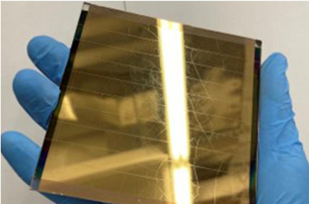
A researcher holds a perovskite module. Credit: Penn State
