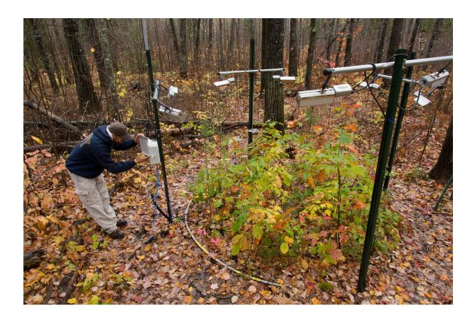
A researcher checks a thermocouple panel (temperature sensors junction box), part of a system that uses heat lamps and soil cables to warm experimental plots at a University of Minnesota field site in northeastern Minnesota. The five-year study, led by University of Michigan forest ecologist Peter Reich, found that even modest climate change may lead to sweeping changes in the northernmost forests, which are called boreal forests. Credit: David Hansen, University of Minnesota.
