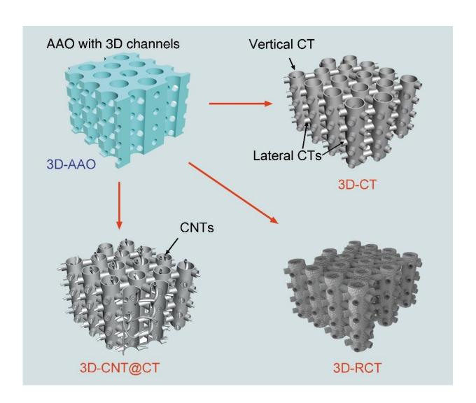
Figure 1. Schematic illustration of the synthesized 3D-CT grids: 3D-CT, 3D-CNT@CT, and 3D-RCT. Credit: HAN Fangming
