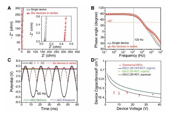
Figure 3. Performance characteristics of single EDLC and EDLCs in series. (A) Nyquist plots. (B) Phase angle vs. frequency. (C) Filtering results of the six EDLCs in series in comparison with AECs. (D) A volumetric comparison of 3D-CT grid-electrode EDLCs with commercial AECs (red triangles, Panasonic, Nichicon, and Nippon, Japan). Credit: HAN Fangming
