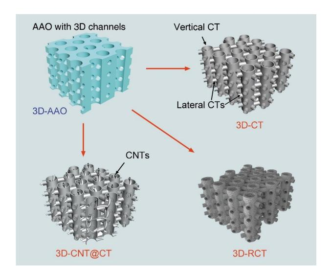
Figure 1. Schematic illustration of the synthesized 3D-CT grids: 3D-CT, 3D-CNT@CT, and 3D-RCT. Credit: HAN Fangming
