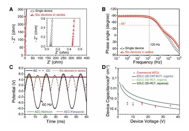
Figure 3. Performance characteristics of single EDLC and EDLCs in series. (A) Nyquist plots. (B) Phase angle vs. frequency. (C) Filtering results of the six EDLCs in series in comparison with AECs. (D) A volumetric comparison of 3D-CT grid-electrode EDLCs with commercial AECs (red triangles, Panasonic, Nichicon, and Nippon, Japan). Credit: HAN Fangming
