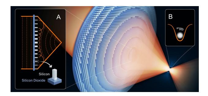
Graphical illustration of light focusing using a planar glass surface studded with millions of nanopillars (referred to as a metalens) forming an optical tweezer. (A) Device cross section depicts plane waves of light that come to a focus through secondary wavelets generated by nanopillars of varying size. (B) The same metalens is used to trap and image single rubidium atoms. Credit: Sean Kelley/NIST
