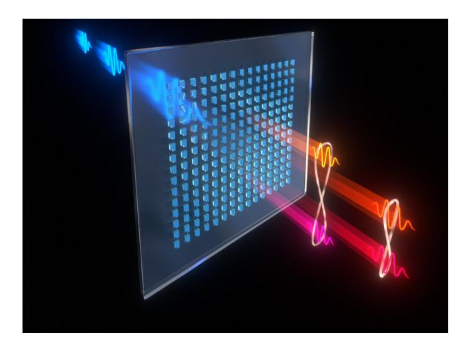
Pump photons pass through a resonant metasurface and produce entangled photon pairs at different wavelengths. Credit: Sylvain Gennaro and Florian Sterl
