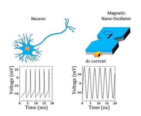
Quantum-materials-based magnetic nano-oscillators provide functionality similar to that of neurons that work via periodic spiking. Credit: The Grainger College of Engineering, University of Illinois Urbana-Champaign
