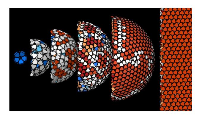
Researchers from Cornell used computer simulations to show how the assembly of vertex-truncated tetrahedra is affected when confined inside a spherical container. The findings offer materials scientists a new method for controlling the assembly structure and characteristics of the resulting material. Credit: Rachael Skye
