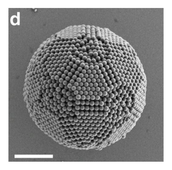
An example of a colloidal cluster from confined self-assembly in a water-in-oil emulsion droplet, a project led by Friedrich-Alexander University Erlangen-Nürnberg. The Cornell simulations could help control the assembly of future colloidal materials. Credit: Wang, J., Mbah, C.F., Przybilla, T. et al. Magic number colloidal clusters as minimum free energy structures. *Nat Commun*
