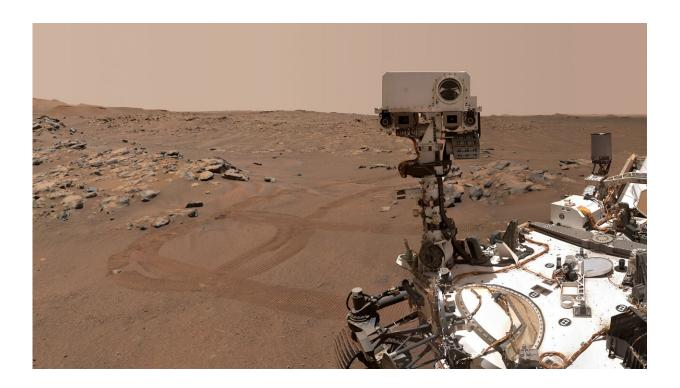
NASA's Perseverance Mars rover took this selfie over a rock nicknamed "Rochette" on Sept. 10, 2021, the 198th Martian day or Sol, of the mission. Two holes can be seen where the rover used its robotic arm to drill rock core samples. Credit: NASA/JPL-Caltech/MSSS.
