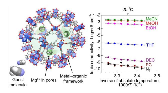
The new Mg<sup>2+</sup> conductor consists of a metal–organic framework holding Mg<sup>2+</sup> ions in its pores. A "guest molecule" acetonitrile is introduced into the structure to accelerate the ionic conductivity of Mg<sup>2+</sup> and allow its migration through the solid. Credit: Masaaki Sadakiyo from Tokyo University of Science
