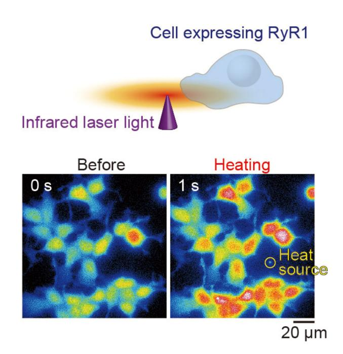
Top, a 1455-nm infrared laser light was focused using an objective lens to apply heat to cells under a fluorescence microscope. The cells expressed RyR1 with mutations that are known to be related to malignant hyperthermia. Bottom,  $Ca^{2+}$
