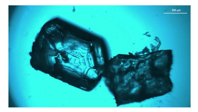
A light micrograph of the linked lanthanide soft crystals used in this study; the dysprosium crystal is on the left and the terbium crystal is on the right. Credit: Pedro Paulo Ferreira da Rosa, et al. *Nature Communications*. July 5, 2022
