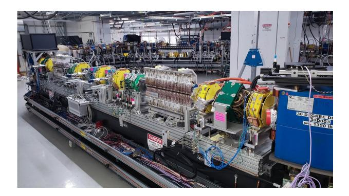
The optical stochastic cooling apparatus occupies the entire 6-meter length of IOTA's long experimental straight. Designed and built by the IOTA/FAST team and industry partners, the system was recently used to achieve the world's first demonstration of OSC. Credit: Jonathan Jarvis, Fermilab
