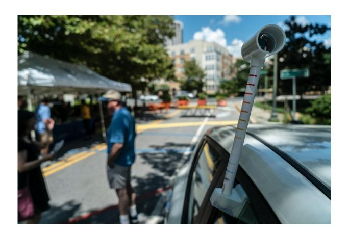
A sensor installed on a car records temperature, humidity, time and location for an urban heat mapping project.
