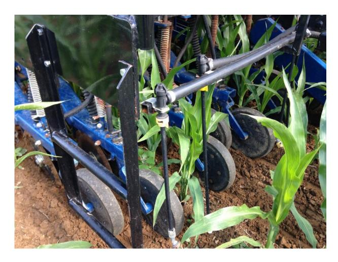
This tool, the InterSeeder<sup>TM</sup> can sow cover crops in between rows in a standing crop like corn. Cover crops are grown to provide benefits to the soil and the environment. They can absorb excess fertilizer, keeping it out of waterways. Credit: Sarah Isbell
