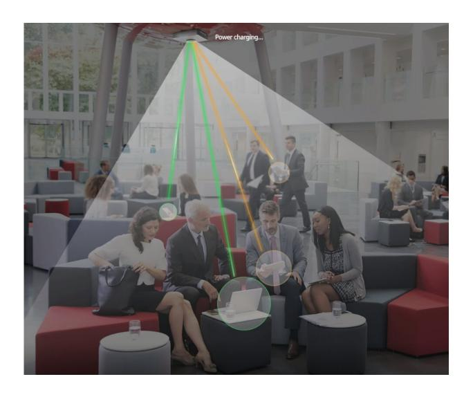
Researchers created a new system that uses infrared light to safely transfer high levels of power over distances of up to 30 meters. This type of long-range optical wireless power transfer system could enable real-time power transmission to fixed and mobile receivers. Credit: Jinyong Ha, Sejong University
