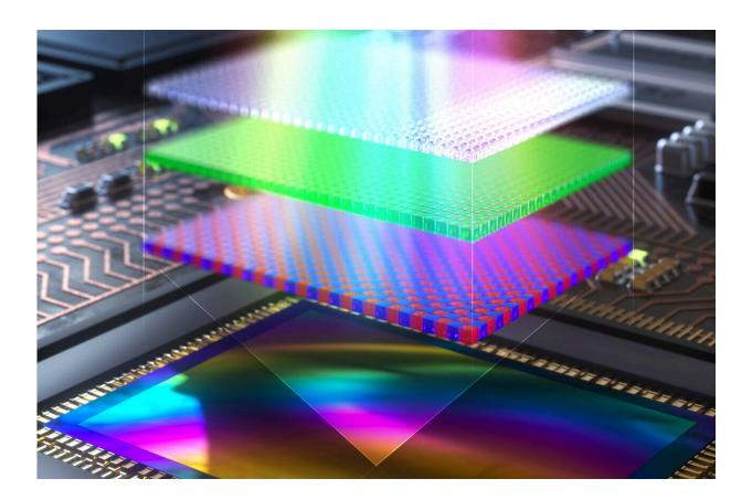
Researchers fabricated green absorbing transparent organic photodetectors that are highly sensitive and compatible with CMOS fabrication methods. They combined one of these green organic photodetectors with a silicon photodiode with red and blue filters to create an organic-silicon hybrid RGB imaging sensor. Credit: Sungjun Park, Ajou University
