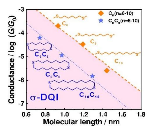
The blue star signs of saturated alkane rings show exponentially decay conductance and the decay trend is similar to saturated alkane chains, which is presented by orange squares. The alkane rings are more insulating than alkane chains when compare the identical molecular length. Credit: Science China Press
