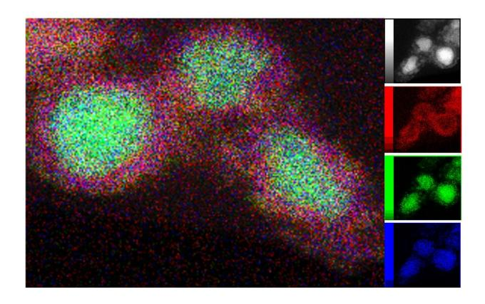
Transmission electron microscopy (TEM) of the catalytically active phase was combined with energy-dispersive X-ray spectroscopy to map the distribution of Ni (green), Si (blue), and oxygen (red) around the core-shell structures. Credit: P. Menezes /HZB/TU Berlin
