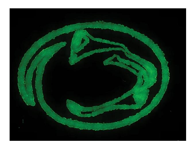
Penn State researchers developed a new nanoengineered granular hydrogel bioink, used here to print an image of the Nittany Lion logo. This bioink helps to achieve previously unattained levels of porosity, shape fidelity and cell integration when 3D printing biomaterials. Credit: Provided by Amir Sheikhi
