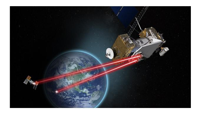
Illustration of LCRD relaying data from ILLUMA-T on the International Space Station to a ground station on Earth. Credit: NASA's Goddard Space Flight Center/Dave Ryan
