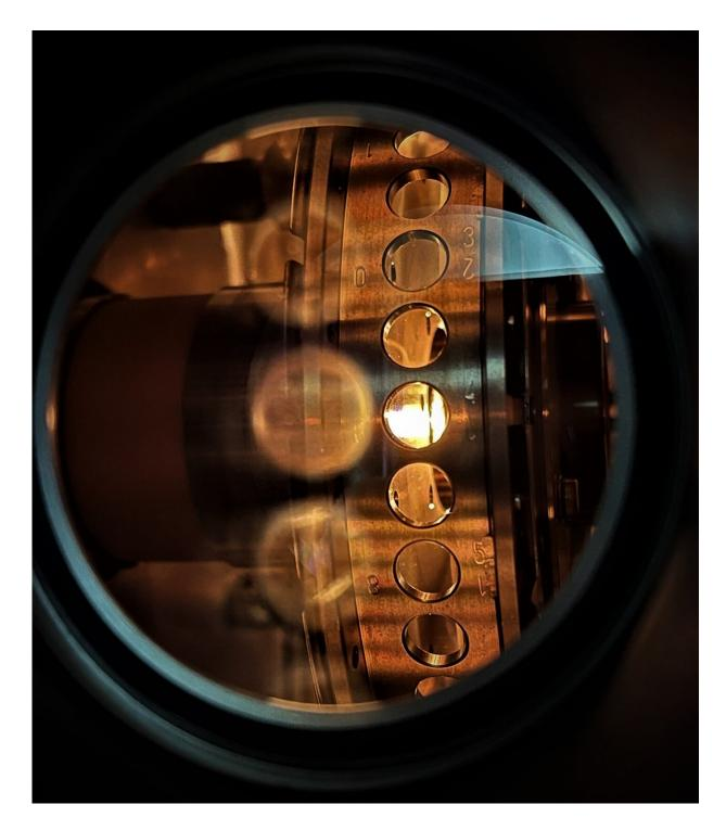
Images of salts of elements being ionized for isotopic measurements in a Thermal Ionization Mass Spectrometer hosted in Ramananda Chakrabarti's lab at the Centre for Earth Sciences, IISc. Credit: Ramananda Chakrabarti
