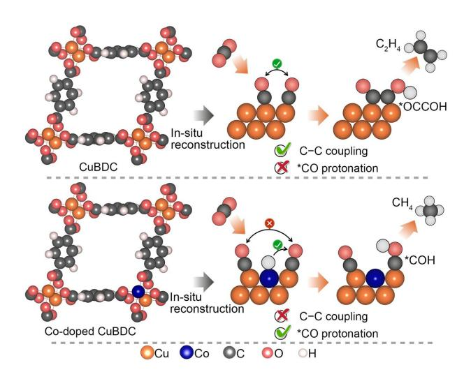
Atomically dispersed Co-Cu alloy fabricated by in-situ reconstruction of the trace-Co doped Cu metal-organic framework is employed as the catalyst for electrochemical  $CO_2$  reduction. The Co dopants in Cu favor \*CO protonation vs. C–C coupling through enhanced \*H adsorption and reduced \*CO coverage, promoting thereby the methane selectivity. Credit: Yang Peng (Soochow
