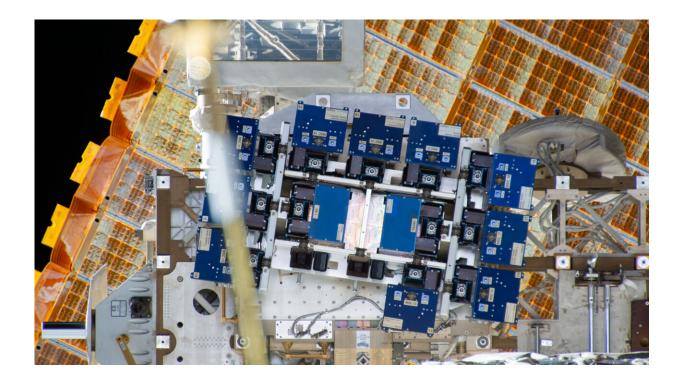
The MISSE Flight Facility on the exterior of the space station. Credit: NASA
