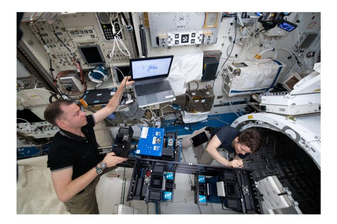
NASA astronauts Nick Hague and Anne McClain install the MISSE-FF inside the Japanese Kibo laboratory module's airlock before depressurizing the unit to move the facility to the exterior of the space station. Credit: NASA
