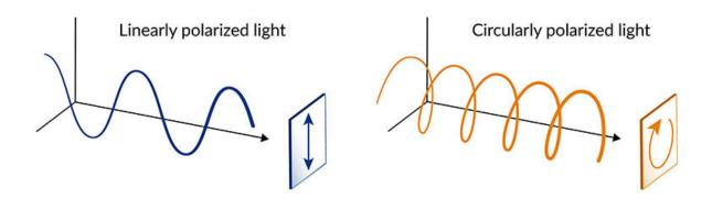
Laser light is usually linearly polarized, meaning that its waves oscillate in only one direction—up and down, in the example at left. But it can also be circularly polarized, at right, so its waves spiral like a corkscrew around the direction the light is traveling. A new study from SLAC and Stanford predicts that this circularly polarized light can be used to explore quantum materials in ways that were not possible before. Credit: Greg Stewart/SLAC National Accelerator Laboratory
