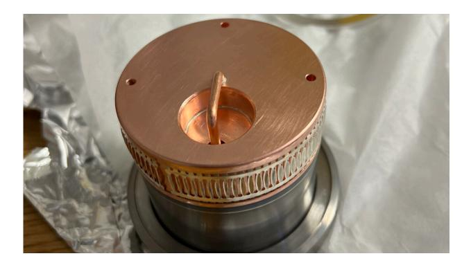
This remade chopper coupler for the Continuous Electron Beam Accelerator Facility came together with the help of a team of experts assembled from across Jefferson Lab. Credit: DOE's Jefferson Lab
