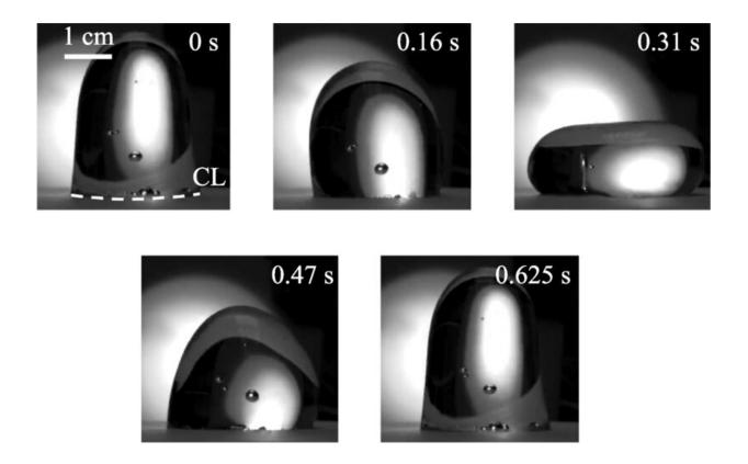
Droplet driven at 1.6 Hz oscillating in the [2,0] mode on substrate F7 exhibits a freely moving contact line. Credit: J. McCraney et al, Physical Review Letters (2022). DOI: 10.1103/PhysRevLett.129.084501
