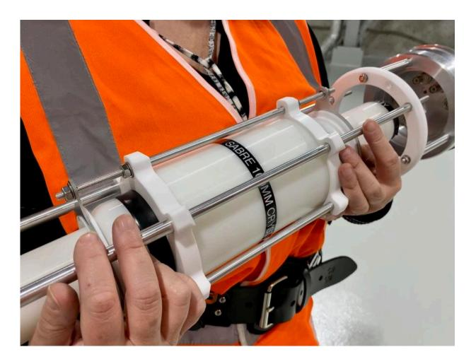
A mock up of the crystal housing cylinder that scientists are using to get used to handling ahead of the experiment. Credit: Imogen Crump
