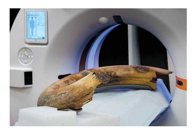
The positioning of the wooly mammoth tusk in the scanner. The tusk was fixed in a fiberglass frame to guarantee transport and table-movement stability. Credit: Radiological Society of North America
